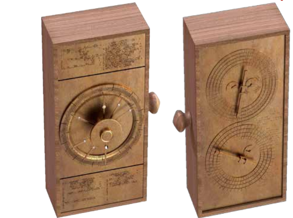
A reconstruction of the Antikythera Mechanism. The front (L) shows the Moon, Mercury, Venus, Sun, Mars, Saturn and Jupiter in the zodiac, with a lunar phase display near the centre. The upper back spiral (R) is a 19-year lunar/solar calendar, and the lower spiral shows lunar months of the 18.2-year Saros cycle in which eclipses are likely to occur. Copyright: Hublot, with fonts from the Aristotle University of Thessaloniki.
